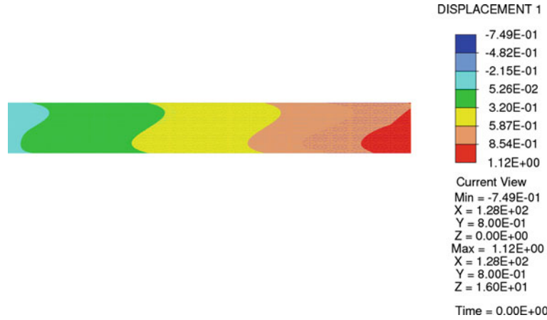
Fig. 2 The distribution of displacement in the x -direction in the x - y plane ( z = 0 )
