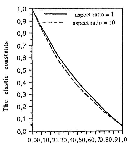
Fig. 7. The elastic constants versus the volume fraction of polymer inclusions
