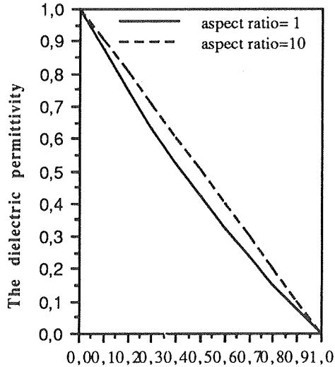
Fig.1. The dielectric permittivity versus the volume fraction of polymer inclusions
