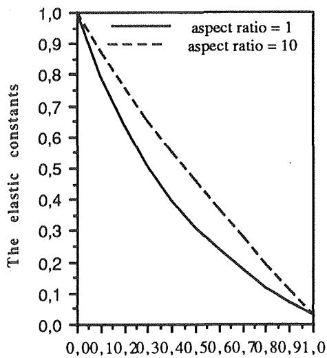
Fig. 4. The elastic constants versus the volume fraction of polymer inclusions
