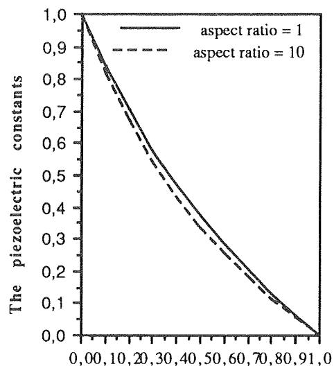
Fig. 10. The piezoelectric constants versus the volume fraction of polymer inclusions
