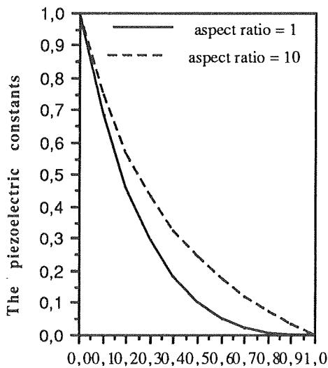
Fig. 8. The piezoelectric constants versus the volume fraction of polymer inclusions
