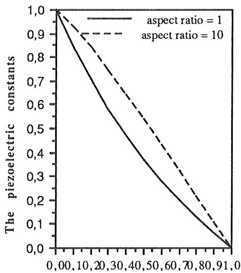
Fig. 9. The piezoelectric constants versus the volume fraction of polymer inclusions
