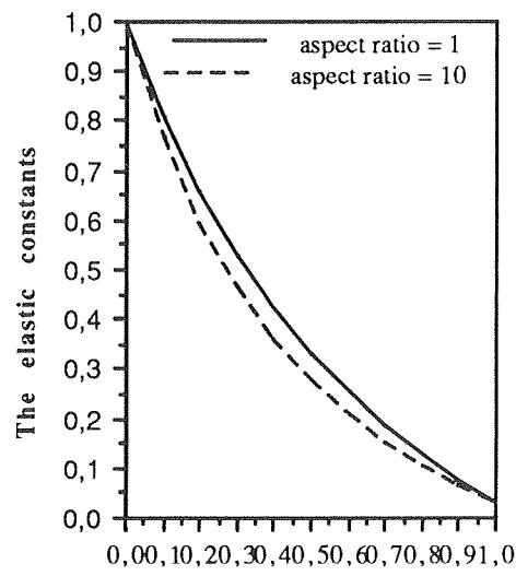
Fig. 3. The elastic constants versus the volume fraction of polymer inclusions
