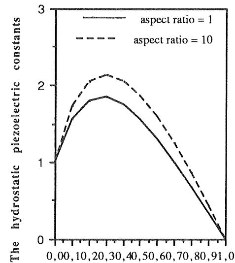
Fig. 11. The hydrostatic piezoelectric constants versus the volume fraction of polymer inclusions
