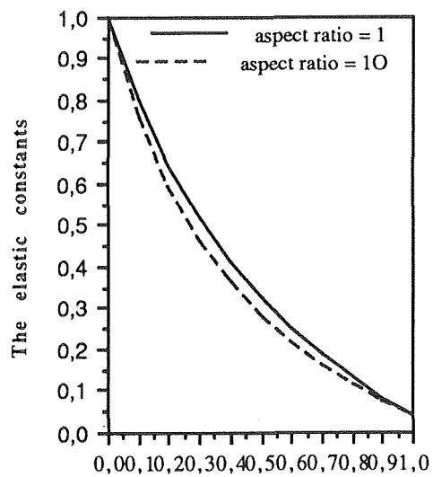
Fig. 5. The elastic constants versus the volume fraction of polymer inclusions
