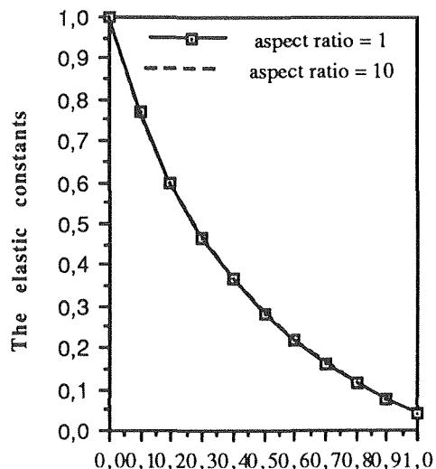
Fig. 6. The elastic constants versus the volume fraction of polymer inclusions
