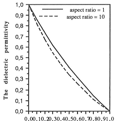
Fig.2. The dielectric permittivity versus the volume fraction of polymer inclusions
